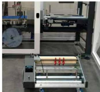
Extractable film dispenser unit. For easy film threading & quick change. Machine can optionally work with center folded and Flat film.
