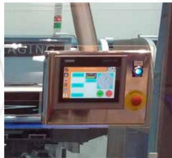
Touch screen intuitive and for easy change of format. Touch screen can rotate in 3 positions. Operator can operate and access the machine from the FRONT/BACK & SIDE. Machine is left/right.
