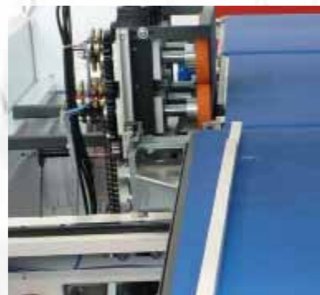
Reduced space between the side sealing and the product, to save 10 cm of side film.
