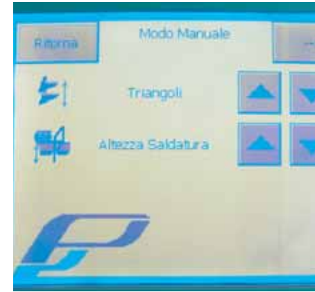
Easy change of format: center sealing and triangle-inverting head motorized. Height up to 400 mm.
