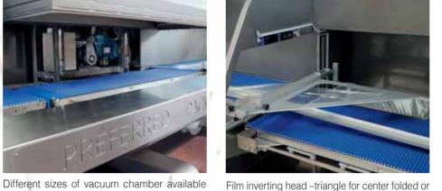
flat film . NO premade bags. Machine works in line with film roll. High versatility and film costs
