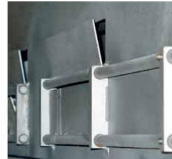
The flaps could be opened and also adjustable for a best ventilation, accordingly the best shrinking.
