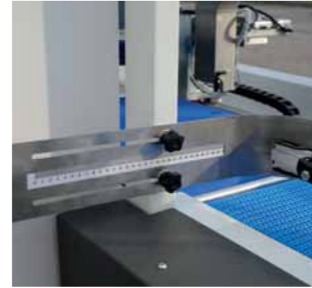
Fast change of format, sizes indicated on the metric line.
