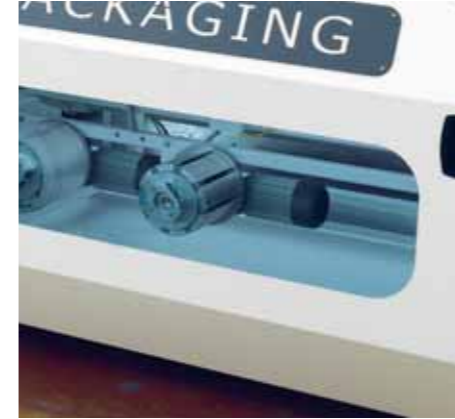
Double dispenser unit for cartons rolls. Optional: handles on rolls.
